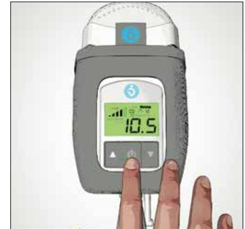
**IMPORTANT:** The “REMINDER” indicator will display on the Z1 if an air leak is detected between the Z1 outlet and the mask. This may also display at times when the mask is not being worn properly. This common condition should clear once all connections are secure, the mask is properly worn, and therapy has begun.
